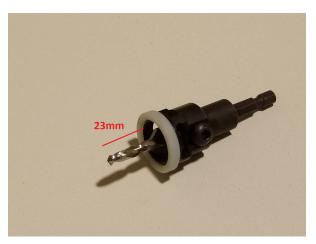
Drill bit length for 19mm thickness decking: 23mm
